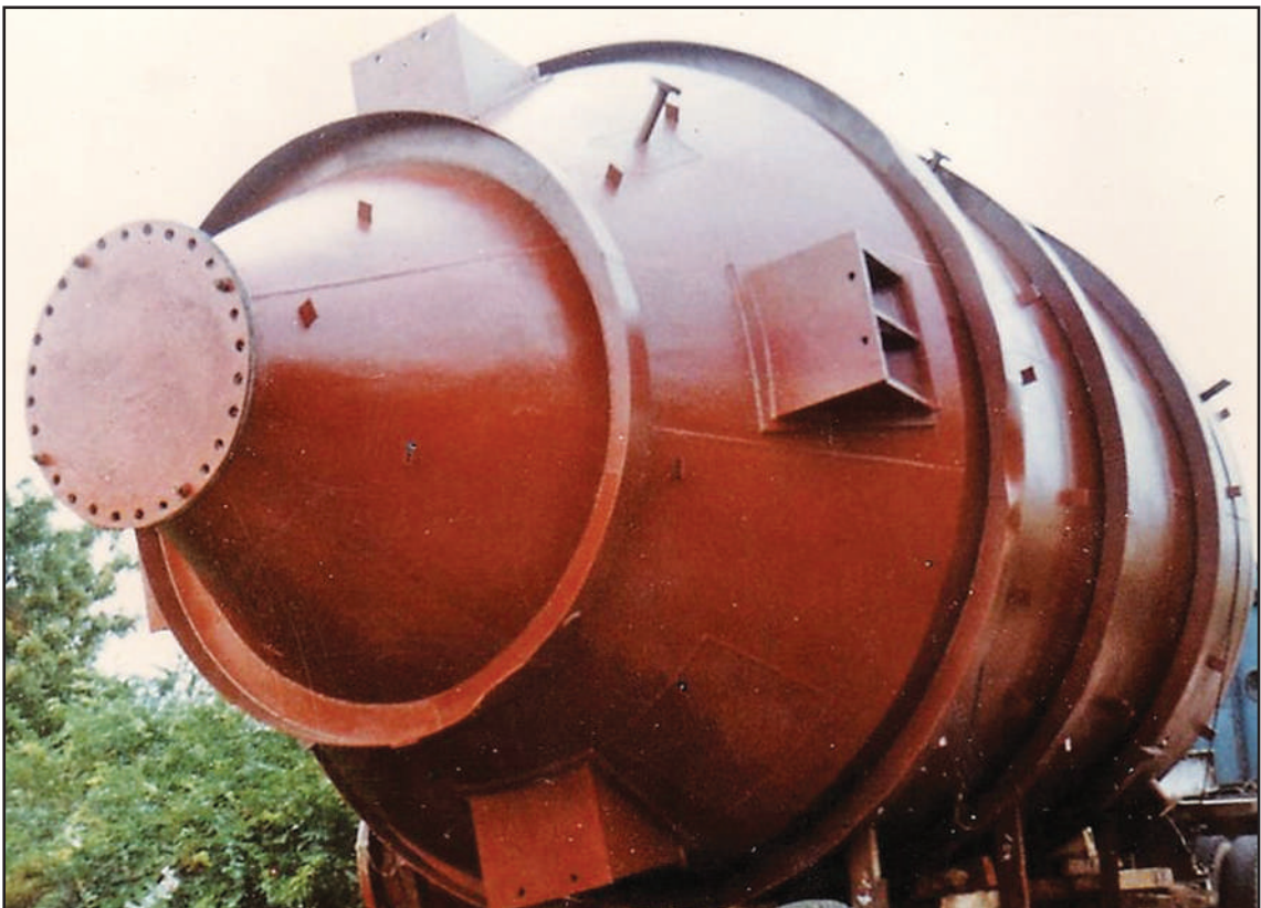
Rubber Lined Flash Chamber
